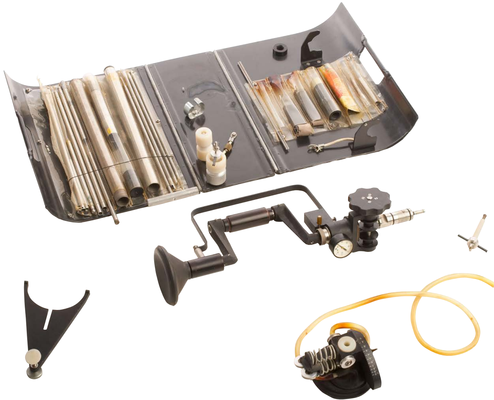
026-BB-HCAD “BELLY BUSTER” HAND-CRANK AUDIO DRILL CIA used the “Belly Buster” drill during the late 1950s and early 1960s. It would drill holes into masonry for implanting audio devices. After assembly, the base of the drill was held firmly against the stomach while the handle was cranked manually. This kit came with several drill bits and accessories.
